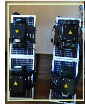
Photovoltaic panels with sunlight simulation
